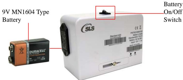
2. **Using SLS Meter Emulator or SMETS2 Electricity Meter** - Connect TSCH STANDARD 420 on ICHIS connector of the meter.
